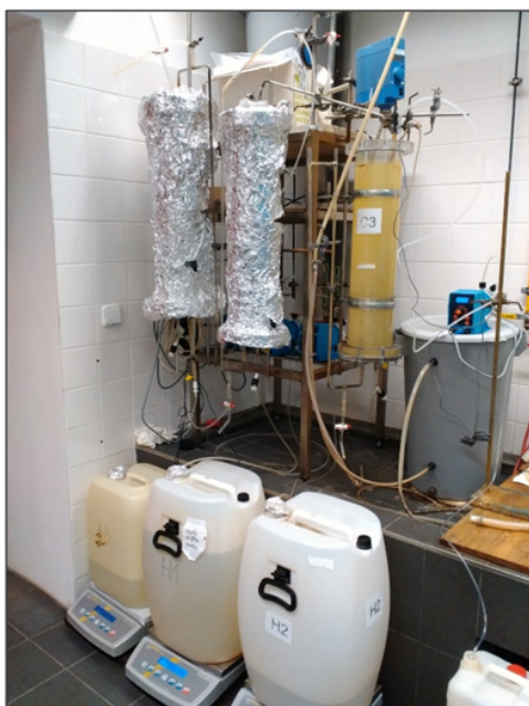
A view of the apparatus in the arrangement for precipitation of metal ions
